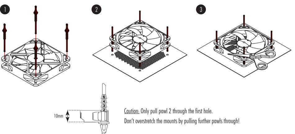
Then pull the C side through the mounting holes of the case. If the long ends of the mounts are in the way, you can use scissors to cut them after installation. Note that this will then make them difficult to reinstall in the future.
