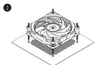
If the long ends of the mounts are in the way, you can use scissors to cut them after installation.
