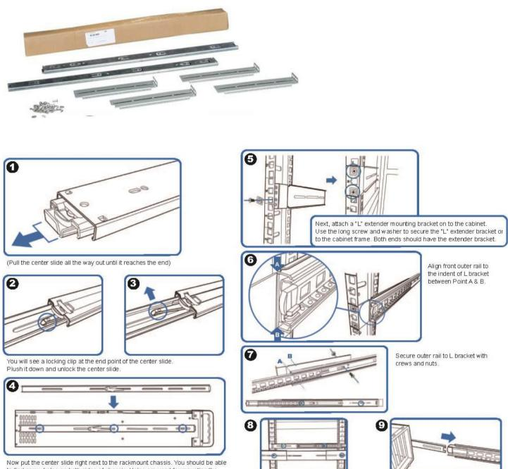
to find screw holes on both sides of chassis. Holes are used for mounting the center slide. Later the center slide will be use for attaching the sliding rail.
