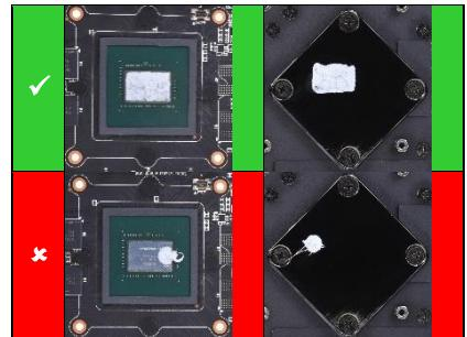
**EN** With the help of a plastic strip or similar spread a thin layer of thermal paste on the GPU. The layer should be less than a millimeter thick, otherwise the surrounding components may be contaminated unnecessarily.
