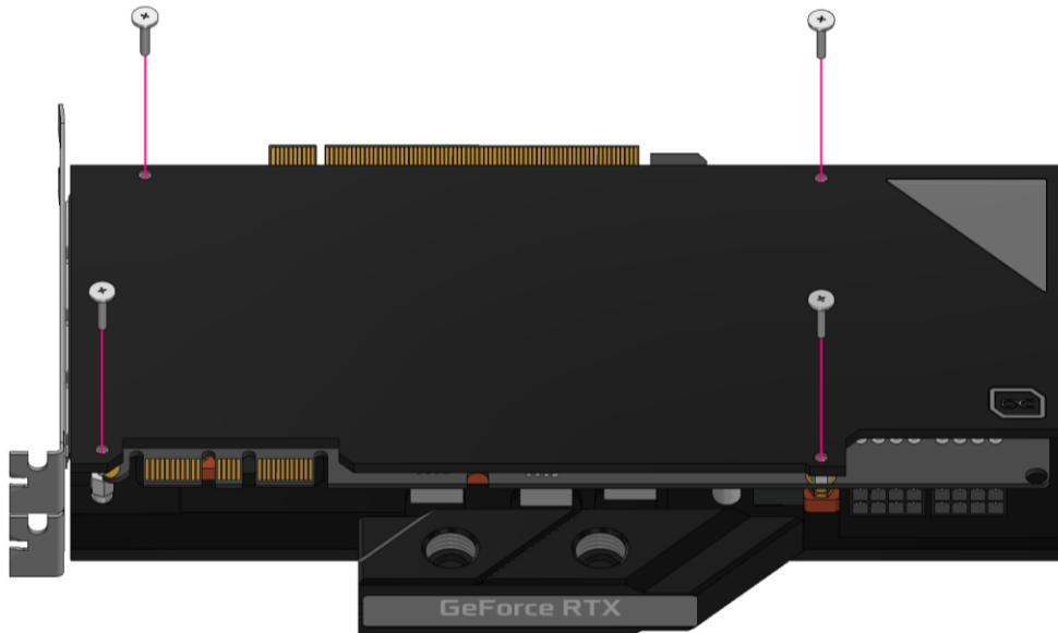
**EN** Put the backplate on and screw it together with the 4 M2x11 screws as shown.
