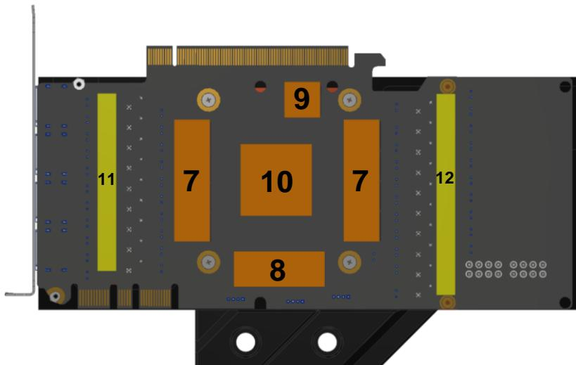
**EN** Remove the protective foils from the thermal pads and place the pads on the PCB as shown.
